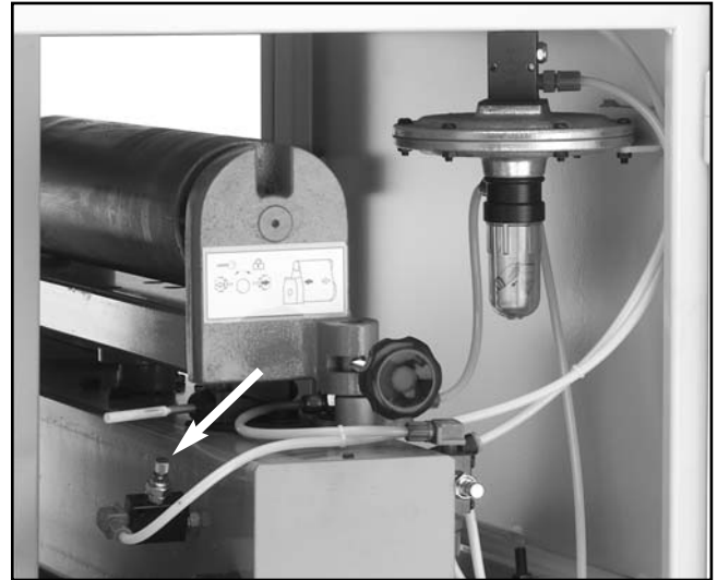
Figure 21. Use the knob on this valve to control oscillation speed.
